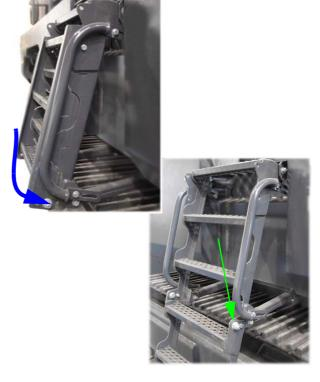
5. Loosen the four fixings on the handles (two either side) and slide out. Tighten the four fixings.
