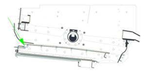
11. Unhook the bottom end of the mesh from the pre-screen.
