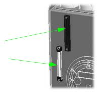
3. If hydraulic fluid is required, remove one of the return filter caps and top up as necessary. Leave the filter in place and fill through the filter.
