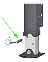
3. Place retention pins in to their storage holders and fit the clips.
