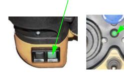
4. Push switch to the left to switch the feeder On and Off.
