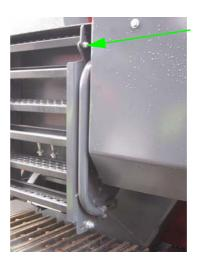
Remove the fixings on the rear ladder and slide the ladder out then secure with the fixing.
