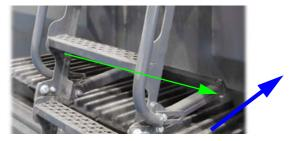
6. Slide the top of the ladder back in to the transport position. Secure ladder back in the transport position.
