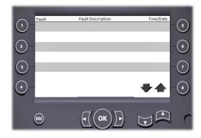
5. Scroll through the fault list using the up and down buttons.
